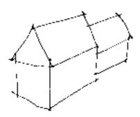
The best approach for an addition to a historic building, Addition is sited at the rear of the original structure and is deferential in size and scale.
