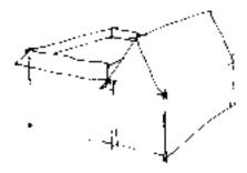
The addition should not compete with the original structure, either in size or location. If an addition must be placed to the side of the historic portion, it should be set back a minimum of 10 ft.
