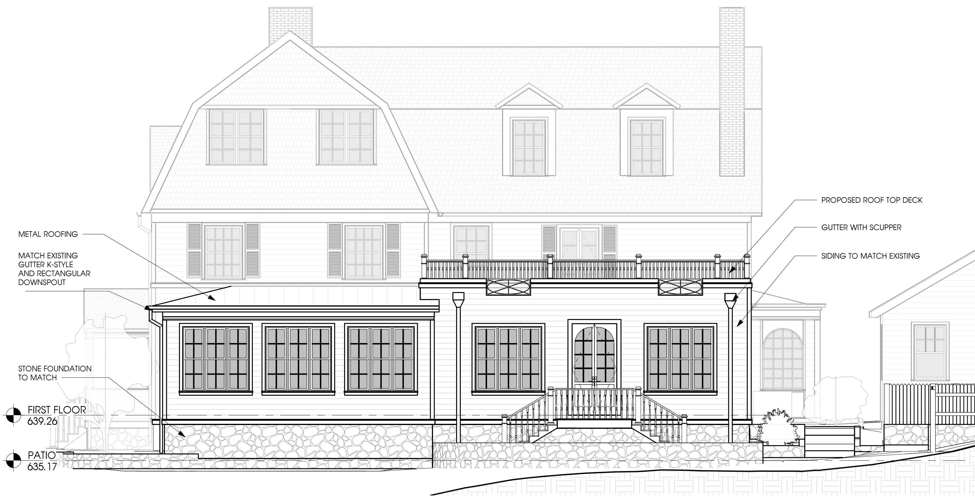
1 PROPOSED - WEST ELEVATION 3/16" = 1'-0"
