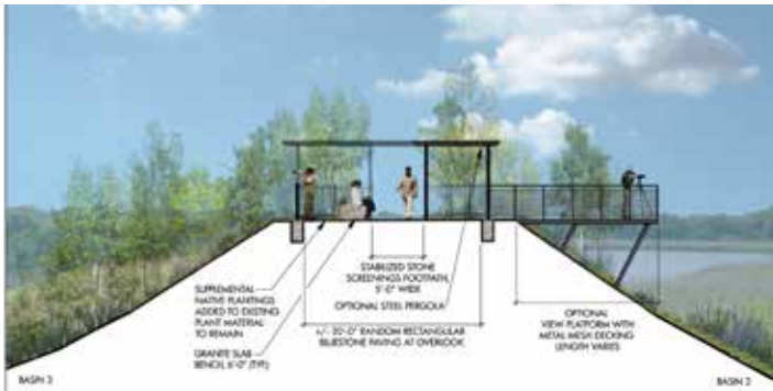
CAUSEWAY PATH BETWEEN BASINS 2 & 3 SECTION-ELEVATION C-C'
