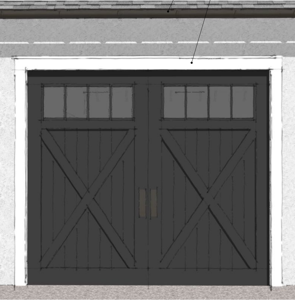
CARIAGE DOORS ALL WOOD CROSS BRACE DESIGN WITH TRANSOM WINDOW PAINTED BLACK TO MATCH FRONT DOOR OF HOUSE
